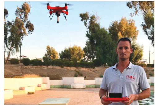
Testing of the observation drone equipped with remote transport and load release devices
