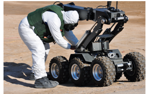
Set up of a mini observation drone on the front platform of a RoV for CBRNE intervention
