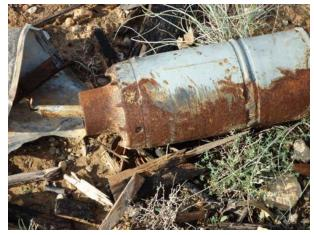
Rupture of the "stand-off" priming device from the shell Source ©M. Guilbaud
