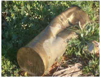
Copper artillery primed case. No propelling charge inside. Only stressed on the outside. source ©M. Guilbaud
