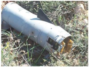
Rupture of the propelling device exposing electronic components. source ©M. Guilbaud
