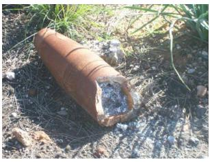
Rupture of the shell body, exposing the inside load to the environment. Source ©M. Guilbaud
